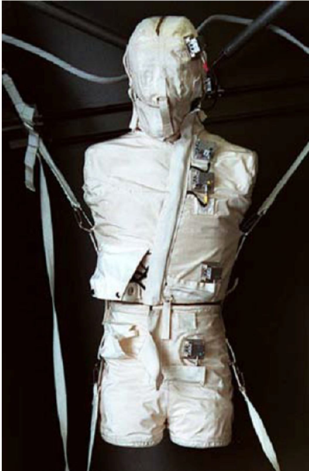
NASA uses an anatomical model of a human torso and head that contains more than 300 radiation sensors.
